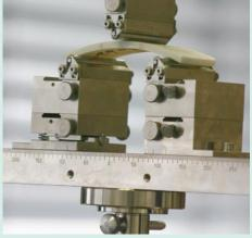
Liner sample undergoing three-point bending test
