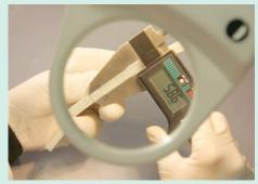
Measurement of liner wall thickness
