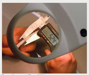
Figure 3: Measurement of liner-wall thickness
