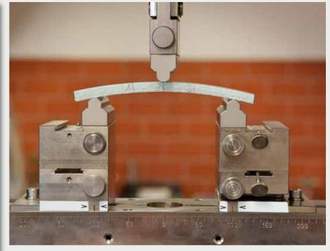
Figure 1: Liner sample undergoing the three-point bendig test
