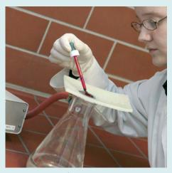
Fig. 3: Examination of the watertightness according to the APS-Guideline
