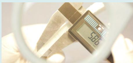
Fig. 2: Measurement of the liner wall thickness
