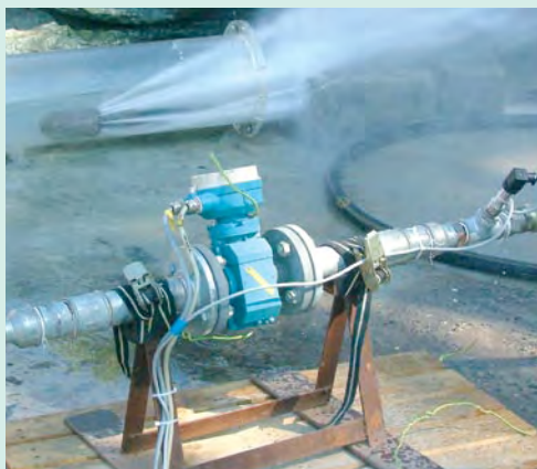
Metrological observation of nozzle pressure and flow rate for exact assessment of test stress
