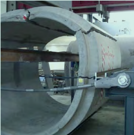
Figure 7: Testing a pipe to failure
