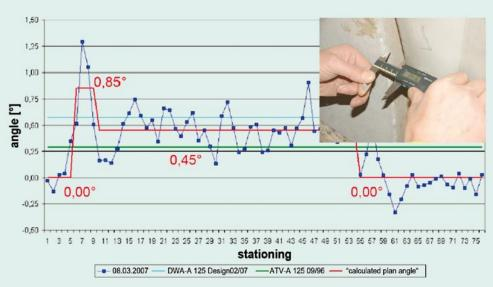
Figure 4 Measurement and corresponding analysis of the joint gap width with a slide rule
