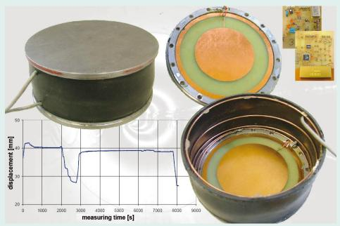
Figure 5 Design of the deformation load cell
