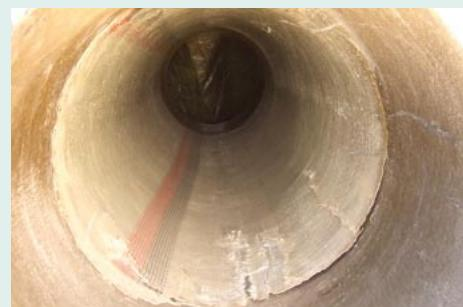
tight repaired points, respectively. The Konudur Sewer Repair Kit (VP) short liners, in which weak points within the GRP laminate resulted in leaks, passed the tightness test up to the highest pressure level only in two of twelve cases. The other three short liners systems tested were all in the mid-range.
