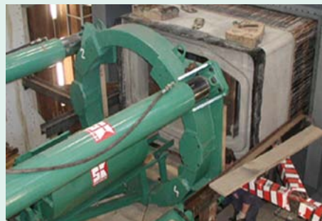
Rectangular jacking pipe: the insertion pit in the IKT large-scale test facility
