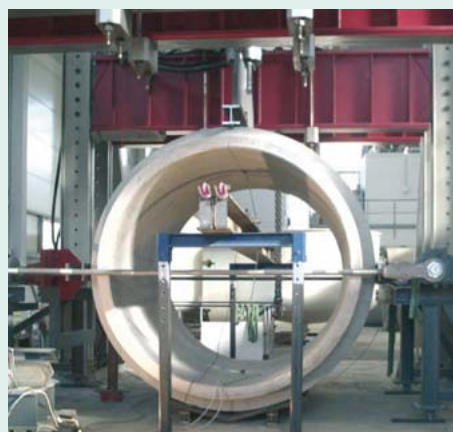
Biaxial compression test (vertical/horizontal) for authentic testing of large-diameter pipes
