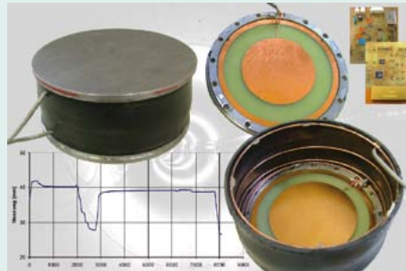
On-line measurement of joint-gap width: measuring instrument
