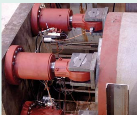
IKT DN 2000 pipe-jacking simulator: jacking pit 8 MN
