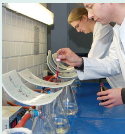
Tightness testing of tube liners
