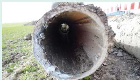
Swollen asbestos-cement pipe in a pressure waste-water conduit
