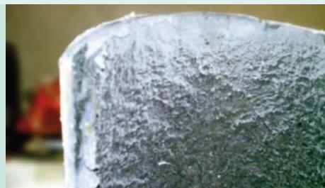
Section from a corroded asbestos-cement pipe in a pressure waste-water conduit
