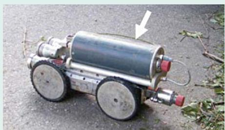
Radar antenna on a camera tractor
