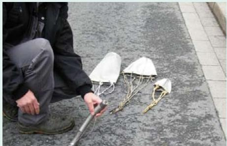
Towed video camera – an axial camera with suction-mount screen
