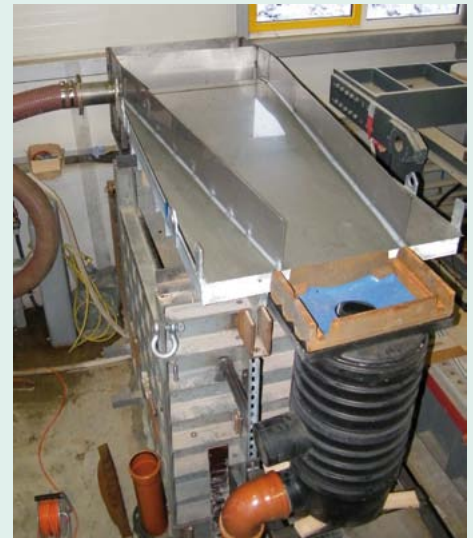
Input of the test apparatus for measurement of hydraulic performance and mass retention
