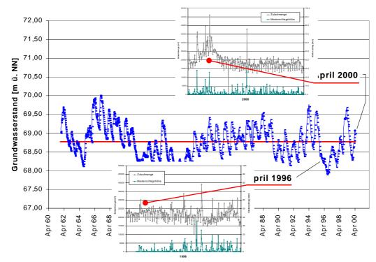
Fig. 2: Long-term fluctuation of the groundwater-level
