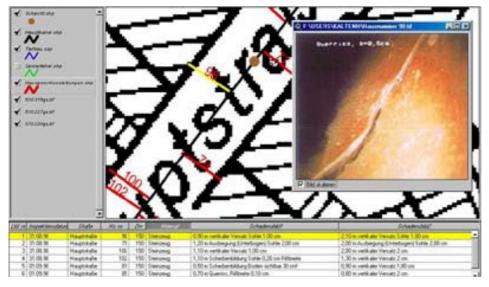
Fig. 5: A Geographical Information System (GIS) supporting the rehabilitation process for private house connections
