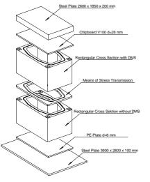
*a)* Basic sketch of the test structureFigure 5 Axial-eccentric load tests
