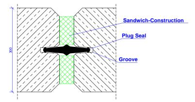
Figure 4 Basic sketch of the sealing system chosen
