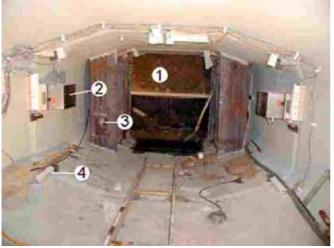
(1) Face (2) Rope distance sensors (3) Target board (4) Distance sensors
