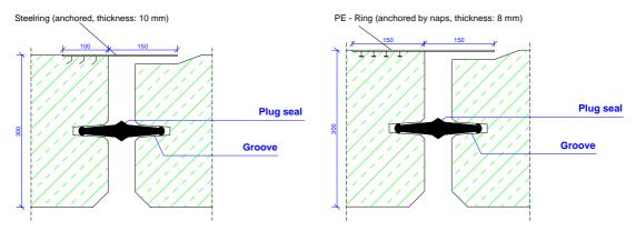
Figure 8 Version of the rings for protection against soil penetration
