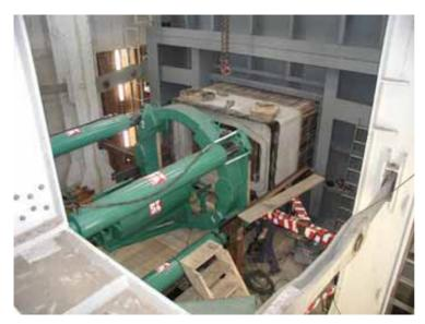
Figure 7 View into the starting pit of the test stand (external dimensions of the pipe 2.6 x 1.85 m)
