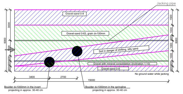
Figure 9 Soil structure for pipe jacking at IKT
