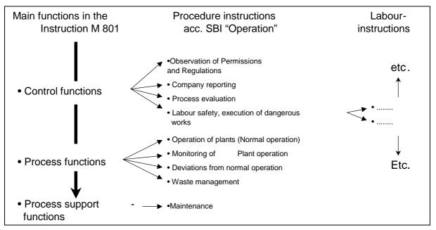
Figure 2: Functions within the Operation Management System
