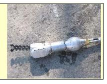
The "Orion L (Kieler Stäbchen)" consists of camera on a pan/tilt head to which a guide bar has been fastened. This is not telescopic. The Orion L is turned into the branching lateral/base line with the aid of the glass fibre rod and enters as it is advanced further. The guide bar always remains in the camera's view during optical inspection.
