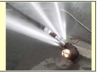
The successor model of the "Göttinger ZK-Kanalwurm 70/500" offers the features of the "old" worm model, while the camera's pan/tilt head also makes it possible, for instance, to pivot over a damage. This model is also fitted with a front rinsing unit, with which the camera lens can be cleaned.
