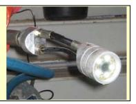
The hydraulically driven "Göttinger ZK-Kanalwurm 70/500" includes a carriage unit with an axial camera mounted in the head of the carriage. The system can be turned up to 90° to the side, and if the "worm" is advanced at the same time, it can be made to turn into lateral/ base line branches. In addition to its function as an inspection unit, the "worm" can be used as a blocking unit for leak tests.
