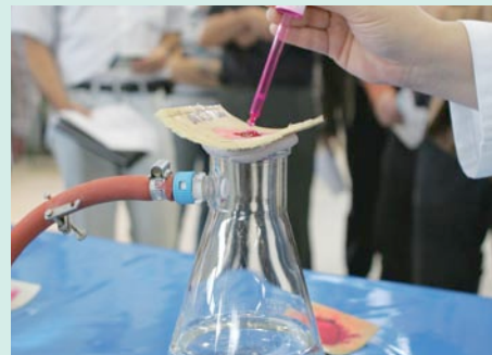
The IKT laboratory: Tightness test in accordance with the APS test and inspection code
