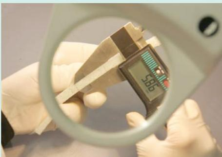
Measurement of liner wall thickness
