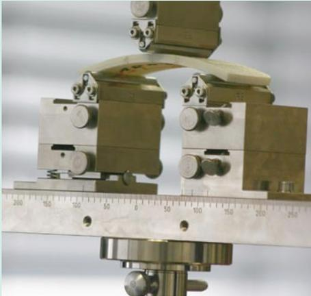
Liner sample undergoing three-point bending test
