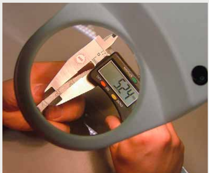
Figure 3: Measurement of liner-wall thickness
