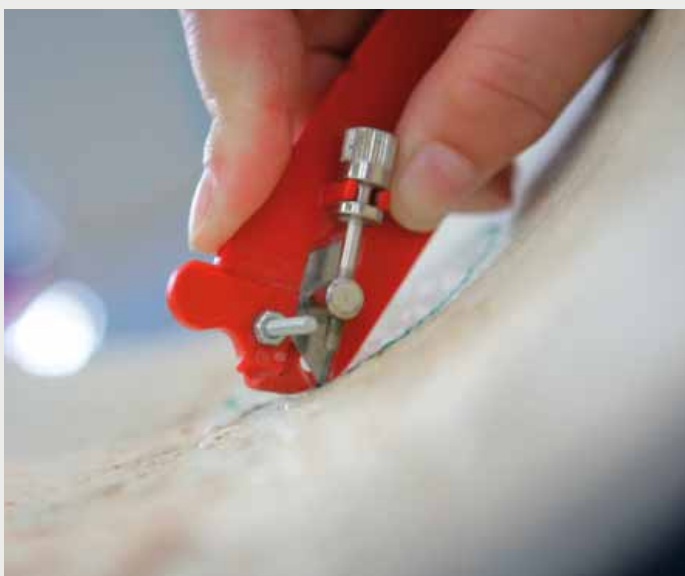
Figure 2: Cut made into inner film, with limitation of cut depth
