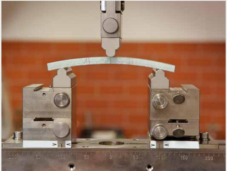
Figure 1: Liner sample undergoing the three-point bendig test
