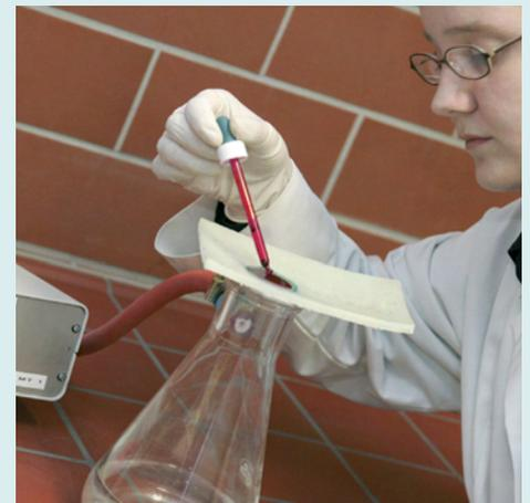
Fig. 3: Examination of the watertightness according to the APS-Guideline
