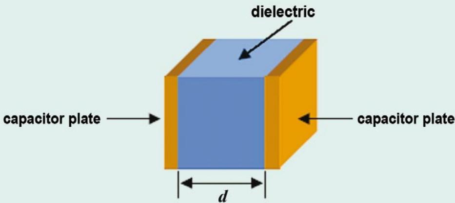
Figure 6 Functioning principle of the deformation load cell
