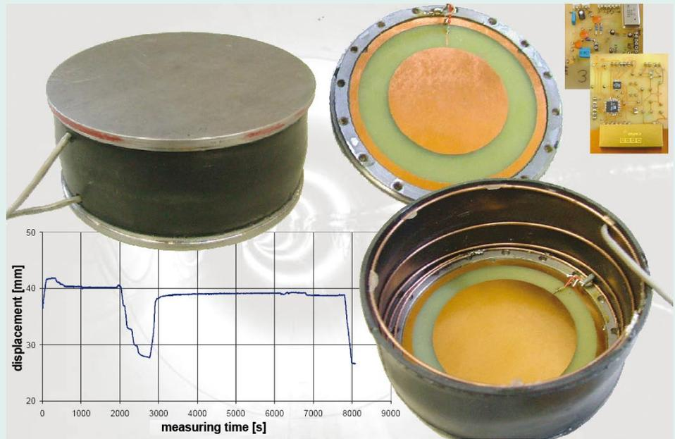
Figure 5 Design of the deformation load cell
