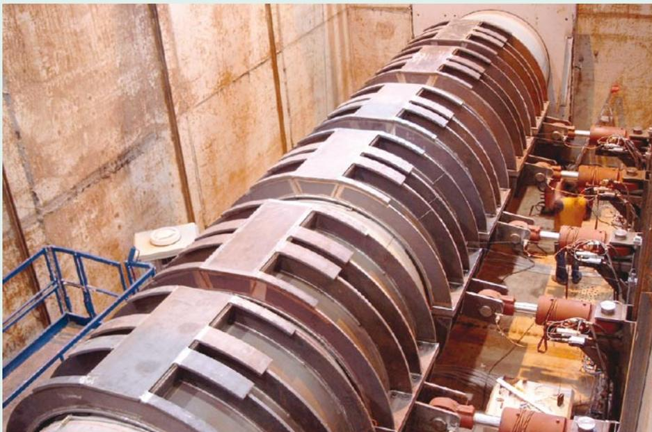
Figure 1 jacking simulator ND 1600 with side hydraulic cylinders
