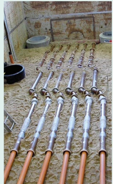
Test lines, extreme situation before covering: different pipe materials and diameter in the IKT large-scale test facility
