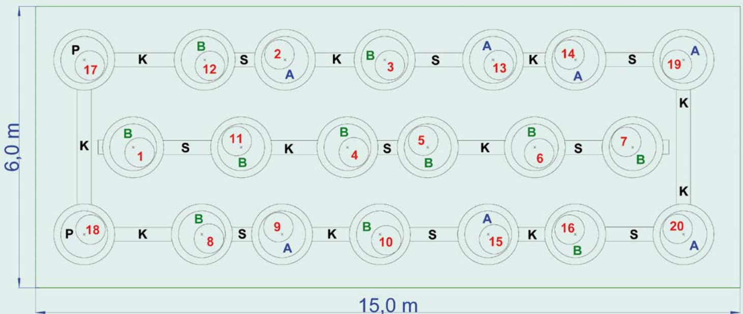
Diagram (plan view) of the manhole structure in the large-scale test facility
