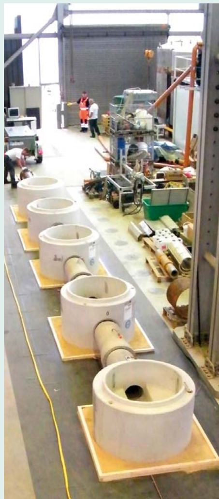
Complex test apparatus: the 12 m long test line in IKT's test shop
