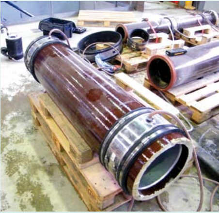
Testing the tightness against external water pressure
