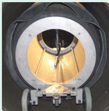
Figure 5: Internal sleeve under test: sleeve on the packer in the conduit
