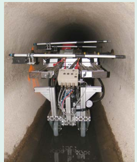
Figure 9: The MAC method: measurements of the system stiffness of the main drain/soil system
