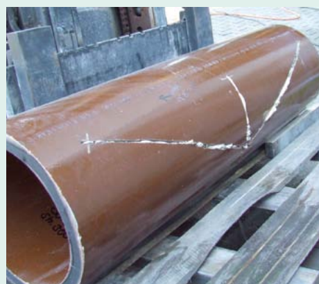
Figure 4: Pressure/grouting method under test: results of the grouting method
