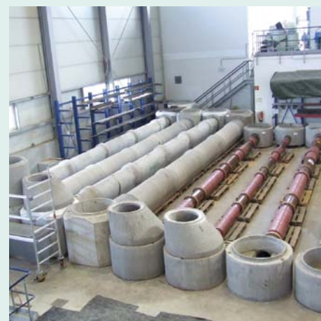
Figure 7: IKT Product Test „Repair methods for DN 200 - DN 600 main drains and sewers“: Test apparatus for short-liners and internal sleeves
