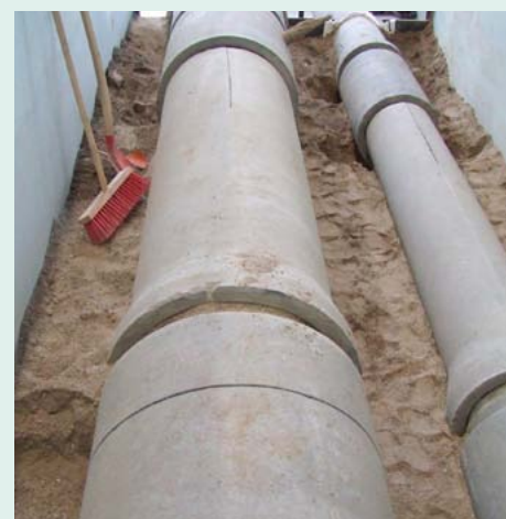
Figure 8: IKT Product Test „Repair methods for DN 200 - DN 600 main drains and sewers“: Test apparatus for injection and grouting/pressure methods
