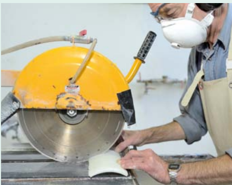
Liner samples are cut to the size and shape needed for testing.
