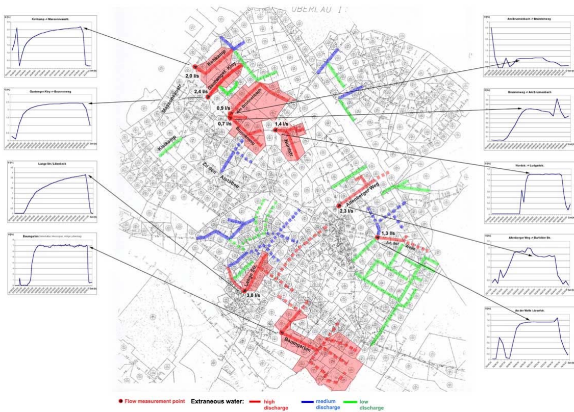
Figure 1: Results of an extraneous water measurement programme (c.f. [5])
