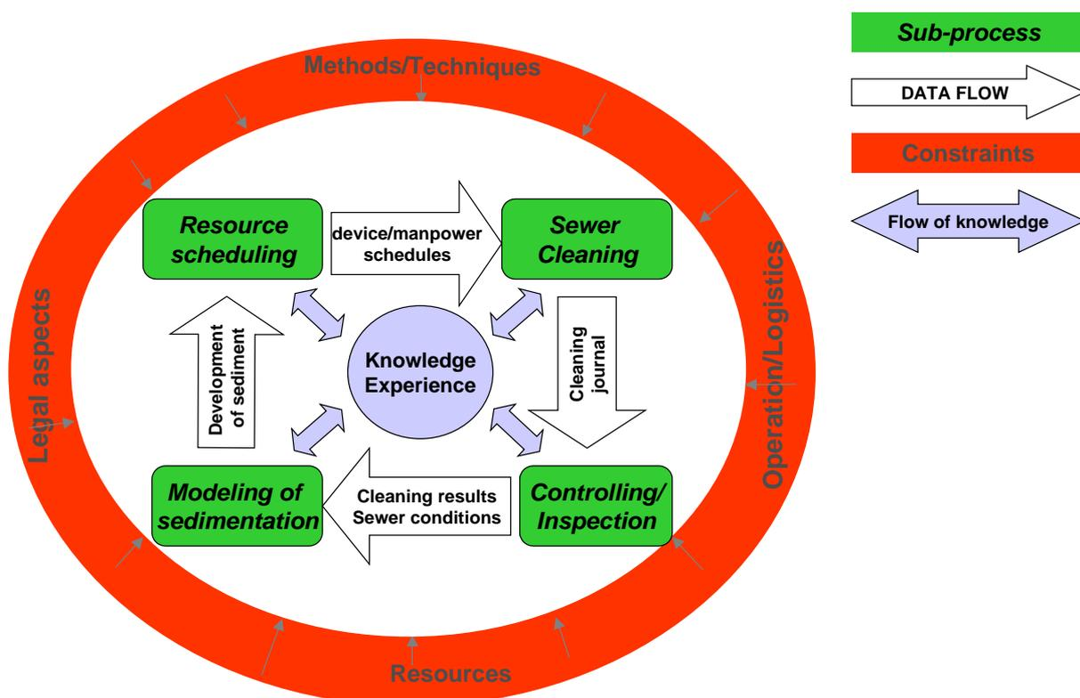
Picture 1: Process: Adaptive Cleaning of Sewage Networks
