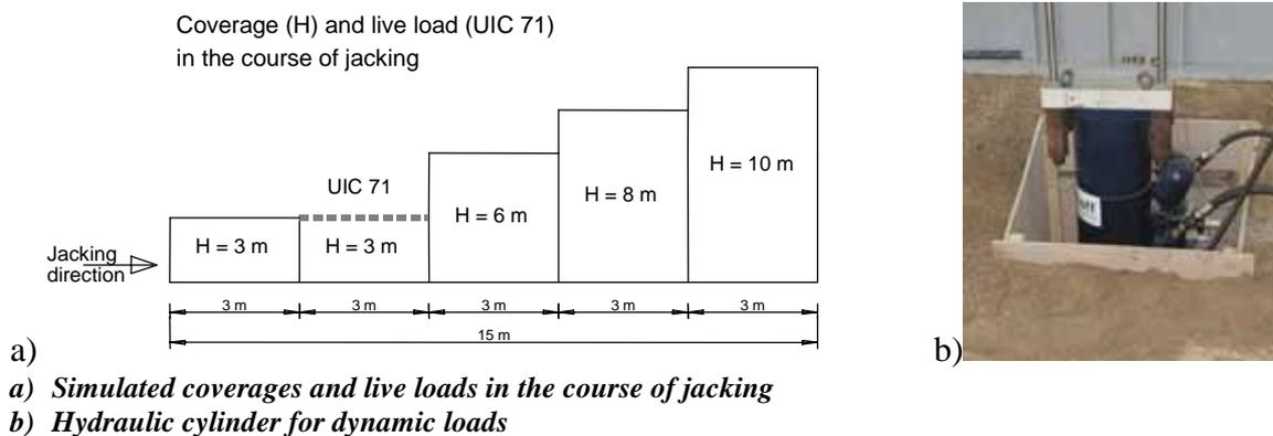
Figure 10 Static and dynamic loads
