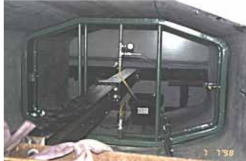
c) Joint test: internal pressure test
