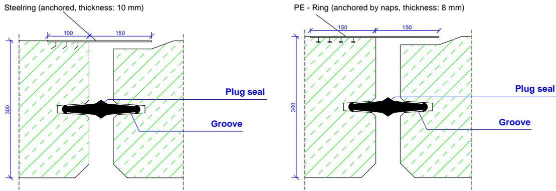
Figure 8 Version of the rings for protection against soil penetration
