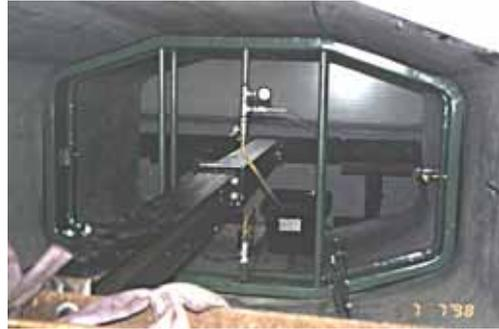
c) Joint test: internal pressure test
