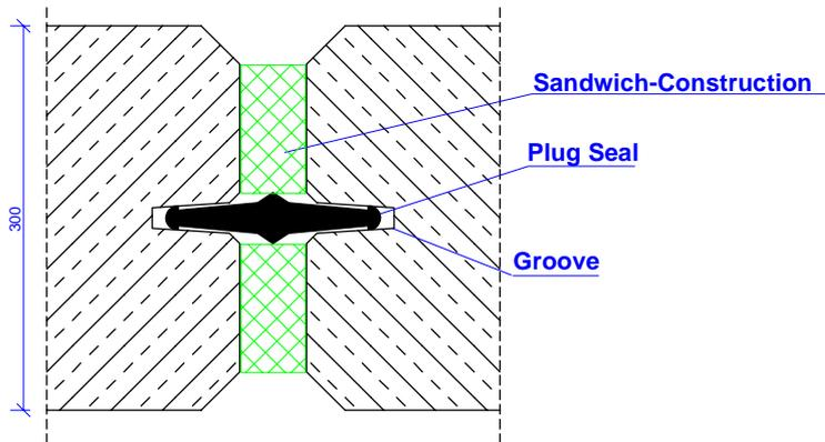
Figure 4 Basic sketch of the sealing system chosen
