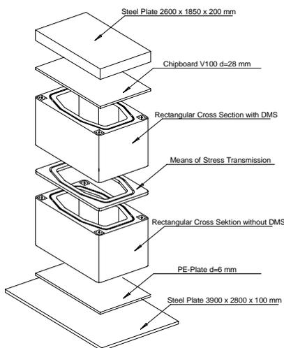
a) Basic sketch of the test structure
