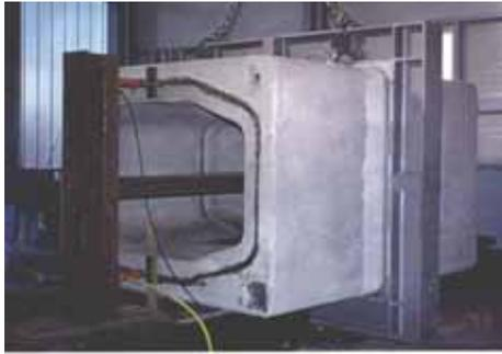
b) Joint test: external pressure
