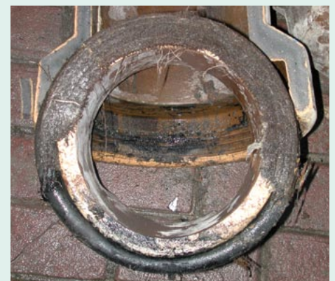
Figure 4 Sealing element of the pipe connection of a combined sewer: Elastomeric ring is covered completely with root cushion in the crown
