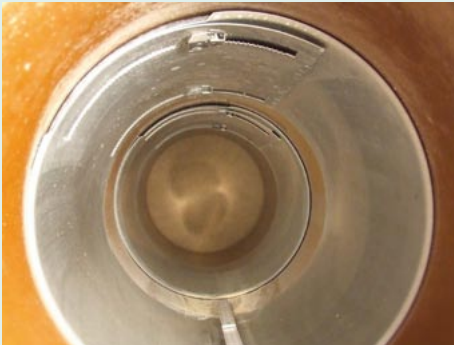
Example of sleeve without (top) and with (down) visible traces of high-pressure flushing
