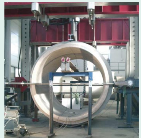
Figure 2 „Modified crown pressure test“ in the multi-axial pressure portal of the IKT [4]
