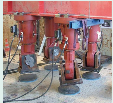
Figure 9: Load transmission for the „Wheel group, static“ load case
