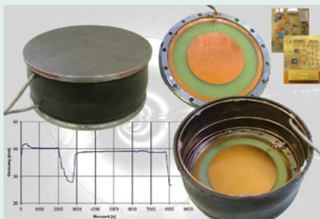
Pipe-jacking: IKT online measurement of pipe offset; above: Radio controlled capsule in on-site use; below: Measuring system setup; from [5]
