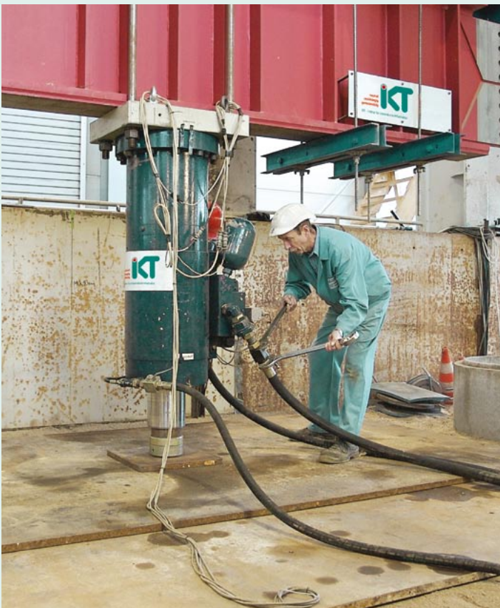
Hydraulic cylinder in the IKT large scale test facility
