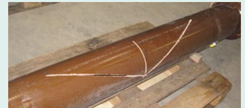
Example of „branching crack“ damage type in vitrified clay pipes
