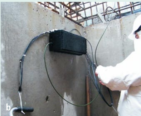
Equipment for temperature measurement a) Cable drum with optical fibre cable b) Connection of the measuring cables on a wall muff in the start manhole
