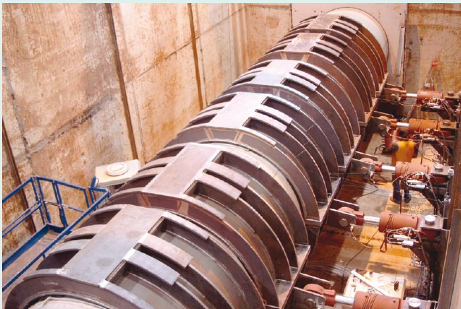
Figure 1 jacking simulator ND 1600 with side hydraulic cylinders
