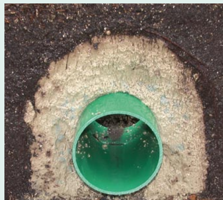
Figure 6 Poplar roots and bentonite body in plant box – roots grow along the boundary area to the bentonite as well as in the bentonite body in isolated cases, from [11]
