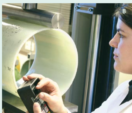
A Adhesive pull test on a coated manhole B Crown pressure test C Flow measurement
