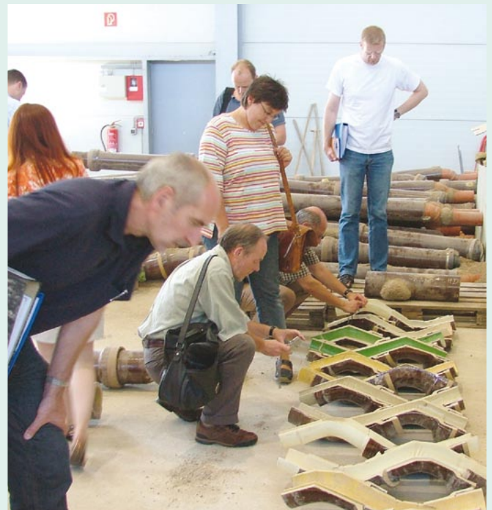
Network operators appraise dismantled testing bodies
