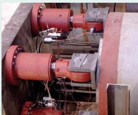
IKT DN 2000 pipe-jacking simulator: jacking pit 8 MN
