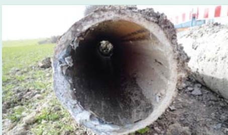
Swollen asbestos-cement pipe in a pressure waste-water conduit (photo: Eastern Holstein municipal alliance)
