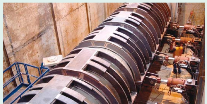
IKT jacking simulator, DN 1600
