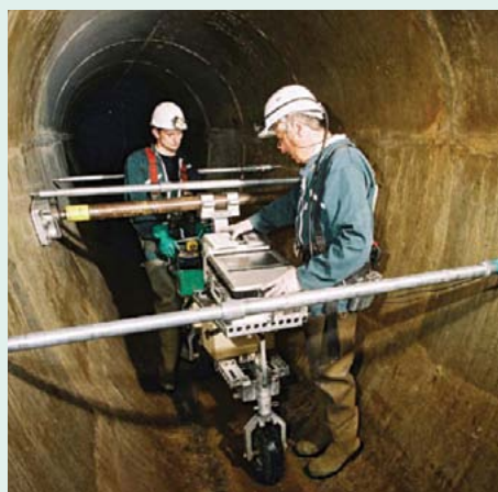
The MAC system (Eau de Paris) for assessment of the stability of large-diameter profiles (photo: Eau de Paris)
