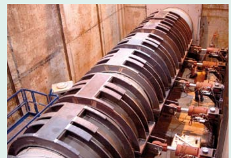
16 m pipe string consisting of five DN 2000 test pipes in a bed structure consisting of positionable steel rings with hydraulic cushions
