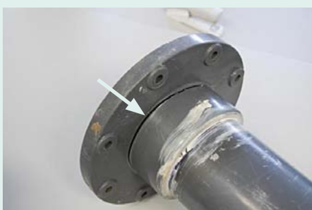
Cracking at a flanged joint in a PVC pressure waste-water pipe at the pumping station (photo: Emmerich/Rhine municipal services)
