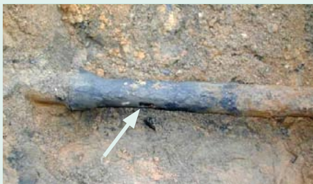
Pitting corrosion in a grey cast iron pressure waste-water conduit (photo: Nuremberg Municipal Drainage and Environmental Analysis Services)
