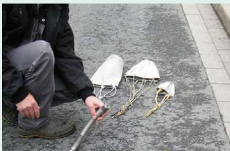
Towed video camera – an axial camera with suction-mount screen
