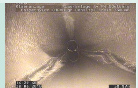
Deformation caused by point load in an HDPE pressure waste-water conduit (photo: Emmerich/Rhine municipal services)
