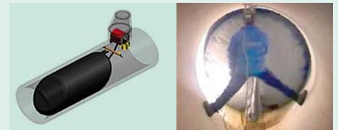
Left: Surge-flushing using the flushing bag: system diagram (HST) Right: in use in the IKT test sewer
