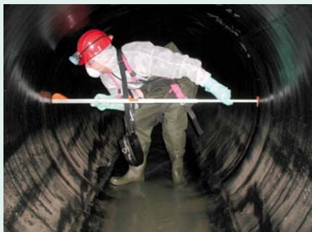
In-situ measurement of deformation in large-diameter plastic pipes
