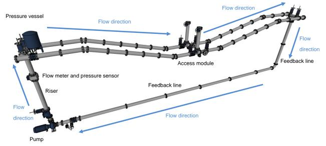
Figure 7. Experimental set up for a pair of test pipes operated separately using a single return line and pump. Blue arrows show the flow direction.
