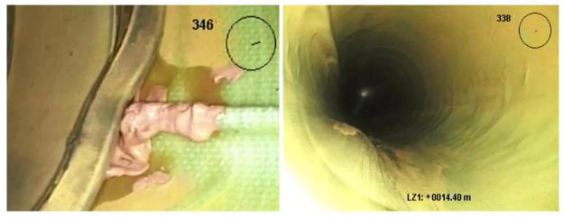
Figure 24. Overall visual impression "Esders HPS Liner": resin seal in the fold area at connection 3 (left), bulge in the liner (right).
