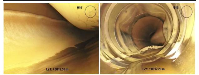
Figure 20. Load-bearing capacity of the "SaniPipe" structure: collapse due to negative air pressure and external water pressure loading.
