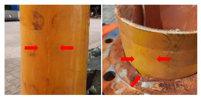
Figure 21. Load-bearing capacity of the "SaniPipe" structure: cracks due to collapse caused by negative air pressure and external water pressure loading.
