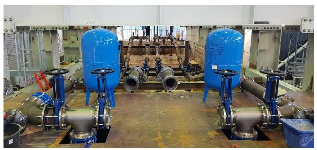
Figure 9. Setup for initial evaluation of the hydraulic performance of undamaged steel pipe, before liner installation (test zero measurement). For pump 1 the continuous undamaged pipe run is on the left side of the test rig and pump 2 on the right side.
