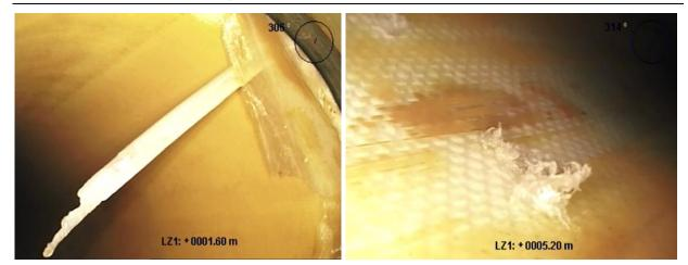
Figure 29. Overall visual impression of "SaniPipe": Damage to end connection after HP cleaning (left), holes in liner after HP cleaning (right).
