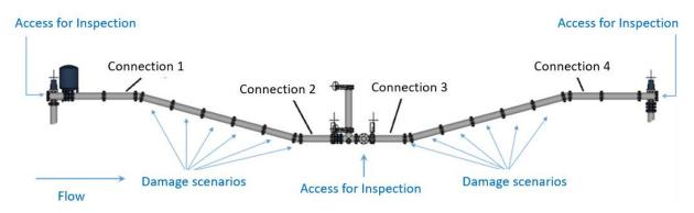
Figure 11. Above-ground test pipeline layout with the location of damage scenarios, access points and connections(end seals). Following installation of a liner the rig contained two sections of liner, each with an end seal at either end: Section 1 between Connections 1 and 2, and Section 2 between Connections 3 and 4. The access module between Connections 2 and 3 was not lined.
