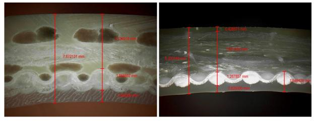
Figure 36. Sectional view: "SaniPipe" (left), "Starline Structure-S" (right).
