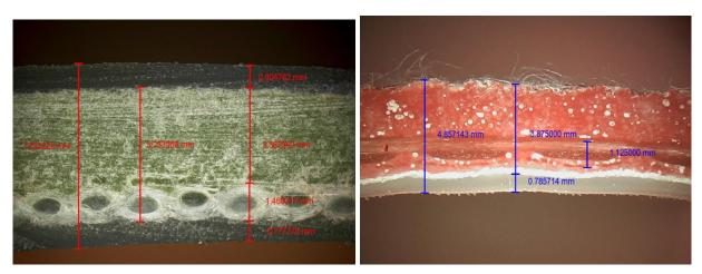
Figure 35. Sectional view: "Esders HPS Liner" (left), "Nordiflow W PE" (right).
