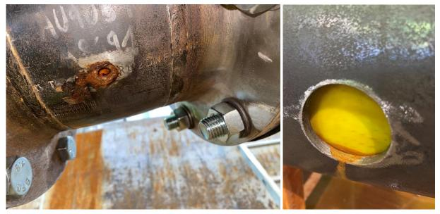
Figure 14 Exfiltration watertightness: Moisture on the "SaniPipe".
