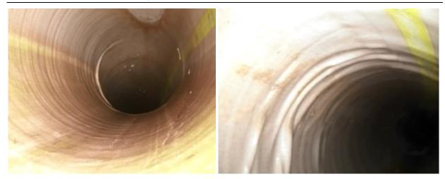
Figure 26. Overall visual impression "Nordiflow W PE": No conspicuous features (left), wrinkles in a bend (right).
