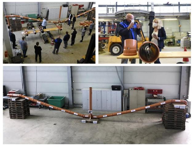
Figure 4. Selection of damage scenarios by the Steering Committee members (top left and right) and the mock test setup in PVC pipe (bottom).
