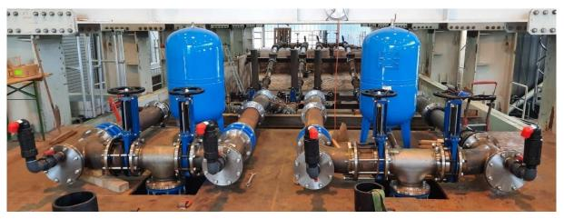
Figure 6. View of testing set-up in the IKT large-scale test facility from the front work platform showing the four installed pipes and blue pressure vessels.
