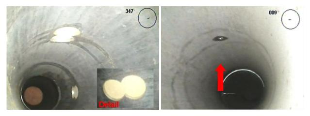
Figure 33. Damage scenario "double ovelapping hole" (left) and shard load, simulated by insertion of a weighted punch through a hole in the crown (F = 300 N, shard punch = ø shank 6 mm/ø tip 2 mm) (right).
