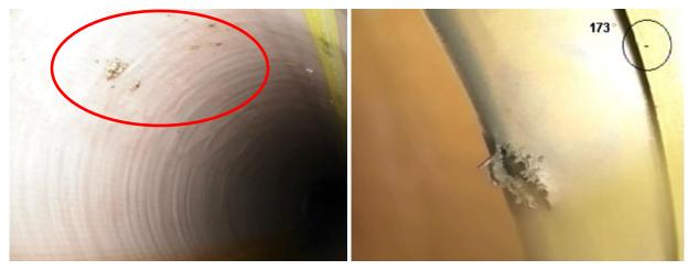
Figure 27. Overall visual impression "Nordiflow W PE": deposits (left), hole in the rubber of an end connection after hig pressure cleaning (right).
