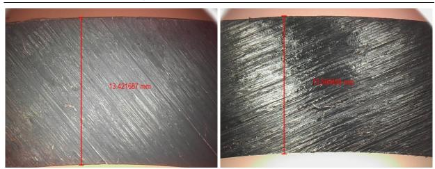
Figure 34. Sectional view: "Compact Pipe" (left), "egeLiner" (right).
