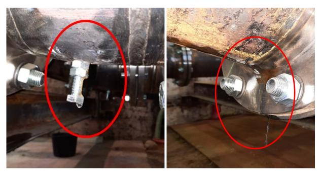
Figure 15. Exfiltration watertightness: Drops on the "Esders HPS Liner".
