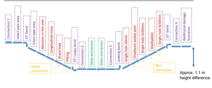
Approx. 19 m width. An additional temporary section of pipe up to a max. 3.3 m added to right, depending on number of additional damage scenarios to be lined
