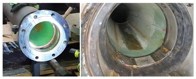
Figure 19. Replacing the sleeves with resin sealant on "Esders HPS Liner": application of sealant (left), rework result (right).
