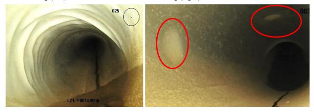
Figure 30. Overall visual impression "Starline Structure-S": wrinkles on a bend (left), discolouration (right).
