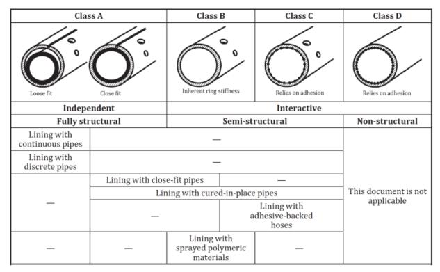
Figure 2. Static classification of lining technologies, from EN ISO 11295 [2].
